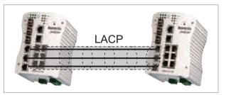
used when you need the wider bandwidth for the backbone network. This is an inexpensive way for you to transfer much more data.
