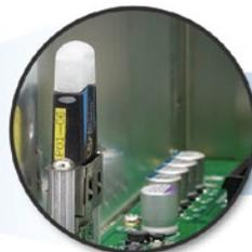
The Matrix internal USB 2.0 port provides increased application security with connectivity for license keys or password encryption on USB dongle.
