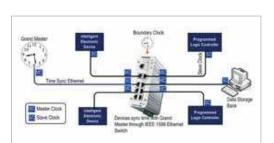
a high level of synchronization within an industrial motion-control environment with a minimum use of network and computing resources. The protocol helps for sequencing event measurements, scheduling outputs, synchronizing actuation, time-stamping, coordinating event records, etc.
