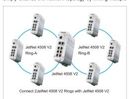
rings into a line or into multiple directions. In addition to extensibility, MultiRingTM has great diversity of various ring technologies. When MultiRing<sup>TM</sup> enabled, JetNet 4508 V2 can connect RSR rings, TrunkRing<sup>TM</sup> and a Super Ring together and simultaneously provide more Fast Ethernet Ring connectivities. This provides extensibility to new technologies while keeping the great backward compatibility.
