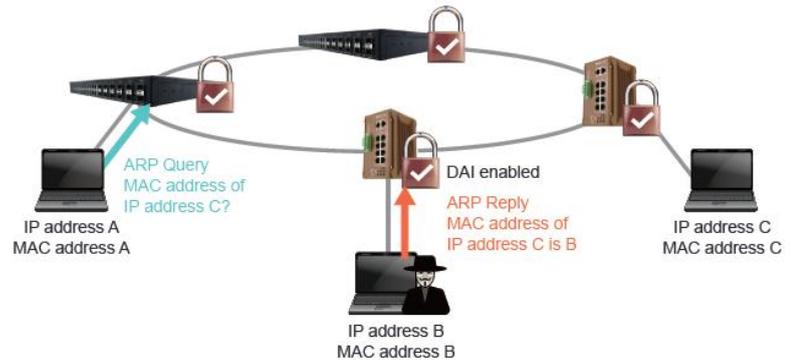
DAI validates the ARP packets in a network. DAI intercepts, logs, and discards ARP packets with invalid IP-to-MAC address bindings. This capability protects the network from some man-in-the-middle attacks.
