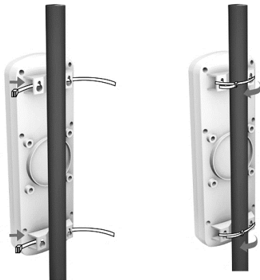
Pole Mounting by using Cable Ties (Default)
