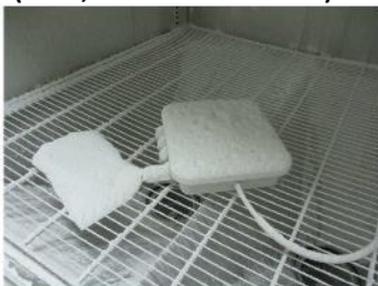
IP6X Dust test (2kPa, 8h duration of test)
