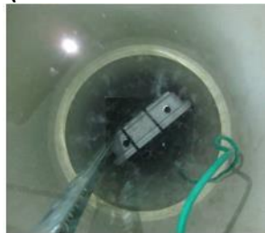
IP7X protection against water (1000mm below the water, 30min)
