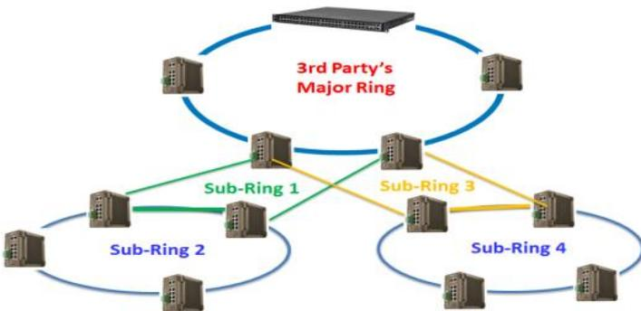
✓ ITU-T G.8032 ERPSv2 reduces coupling Ring failure recovery time
